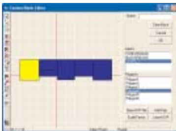
Custom Block Editor - Import floor plans from DXF files produced in a CADD program.
